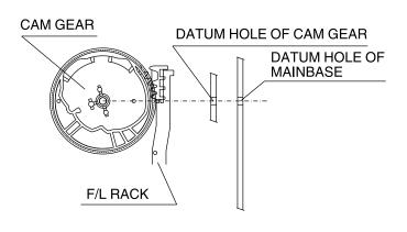
Fig.3-13 ASSBMBLY OF THE CAM GEAR & F/L RACK
